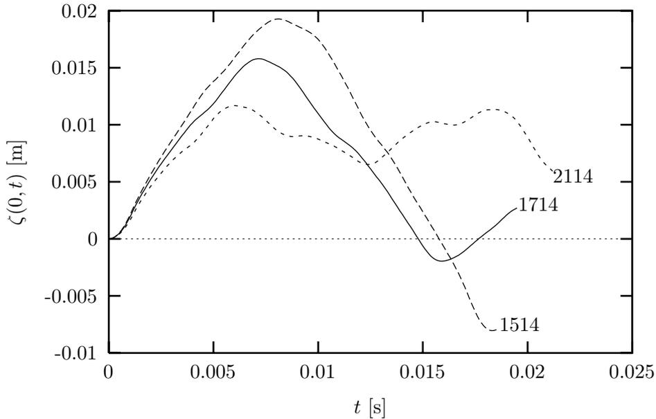
Figure 12: Paths of nock of three different arrows until nock passes pressure point. ( — ) standard arrow 1714X7, ( - - - ) stiffer (and heavier) arrow 2114X7 and ( - . - . ) more flexible (and lighter) arrow 1514X7. Latter arrow slaps against pressure point.
