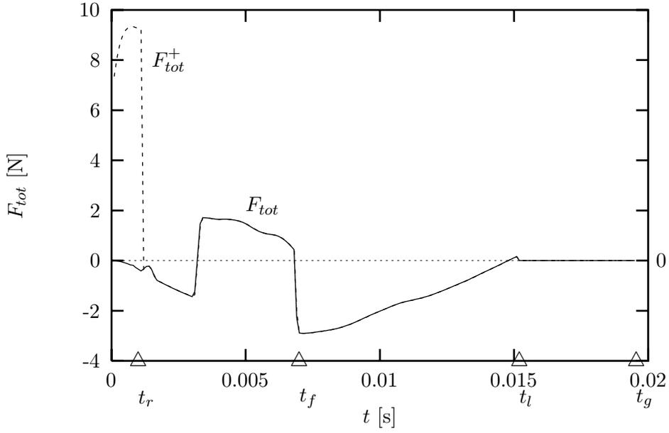
Figure 10: Total force  $F_{tot}$  acting on arrow in  $\zeta$ -direction (13), ( -- ). Also  $F_{tot}^+$ , (14), ( — ), is shown.  $F_{tot}^+ = F_{tot}$  for  $t > t_r$ . Arrow loses contact with pressure point definitely at  $t = t_f$ . Arrow leaves string at  $t = t_l$  and nock passes pressure point at  $t = t_g$ .
