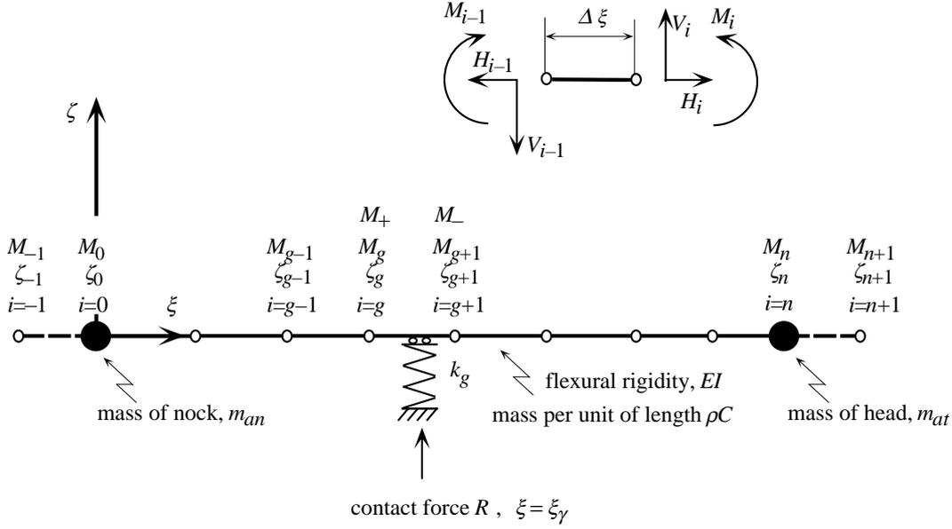
Figure 6: Scheme of model of arrow. Each element,  $i = 1, \dots, n$ , has length  $\Delta\xi$ . Between grid-points we have mass per unit of length  $\rho C$  and flexural rigidity  $EI$ . Two fictitious points outside arrow are introduced, grid-points  $i = -1$  and  $i = n + 1$ . Pressure point at  $\xi = \xi_\gamma$ . Grid point to the left of pressure point is denoted by  $g$ . Two extra unknown bending moments  $M_-$  and  $M_+$  at points  $g$  and  $g + 1$ , respectively.
