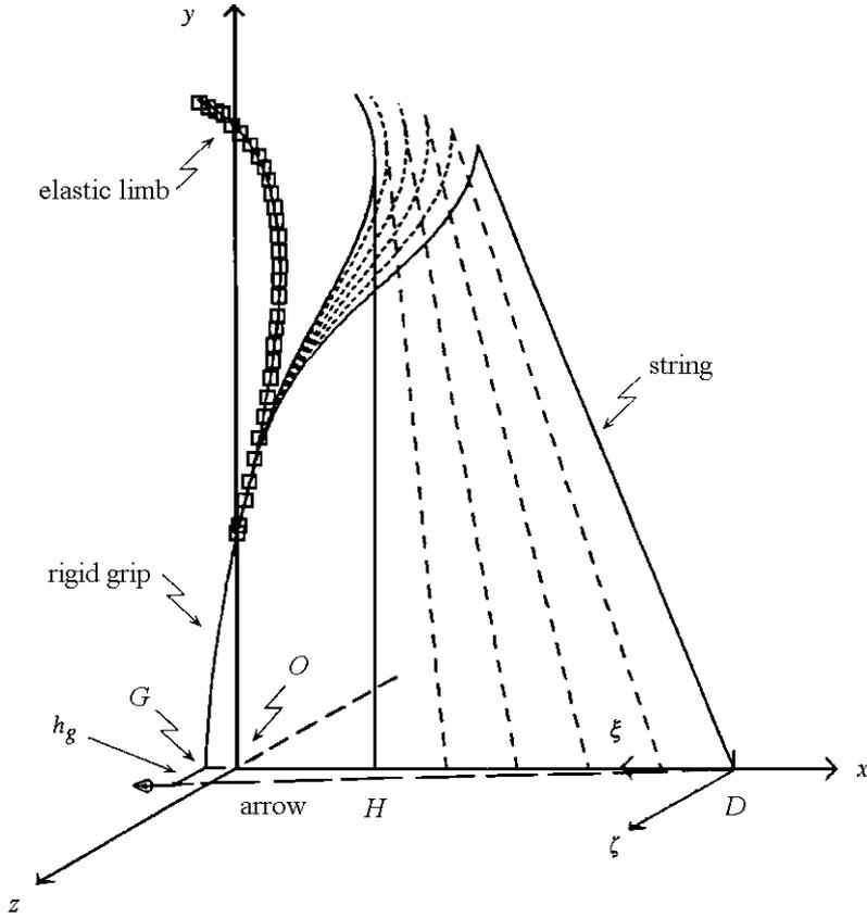
Figure 3: Static deformation of the modern working-recurve bow: the unbraced bow ( $\square$ ), braced bow and fully drawn bow ( $\text{---}$ ) and some intermediate situations ( $\text{- -}$ ). At  $t = 0$  the arrow and the moving coordinate system  $(\xi, \zeta)$ , in which the transverse movement of the arrow is described, are shown.
