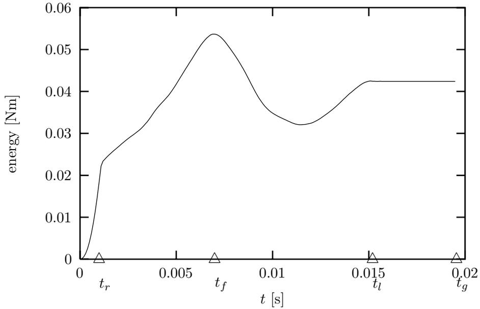
Figure 11: Transverse kinetic energy plus potential bending energy of arrow plus energy in spring which represents transverse elasticity of bow plus energy in spring of pressure button.
