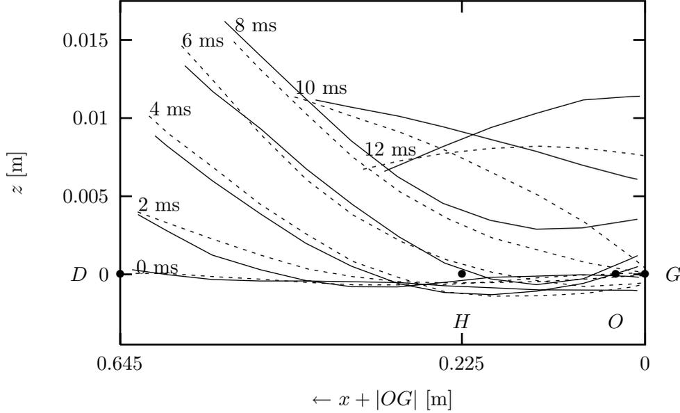
Figure 7: Deformation of arrow: experimental data ( --- ) and calculated by Pękal'ski ( — ), every 2 ms after release, [11]. Only parts of the arrow for  $\xi \in [0, \xi_\gamma(t)]$  are shown.
