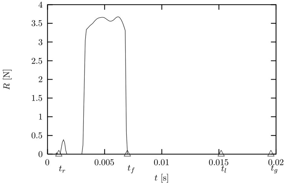
Figure 9: Contact force  $R(t)$ . ( — ) obtained by means of acceleration force  $E(b)$  of Figure 4. Arrow leaves pressure point definitely at  $t = t_f$ . Arrow leaves string at  $t = t_l$  and nock passes pressure point at  $t = t_g$ .
