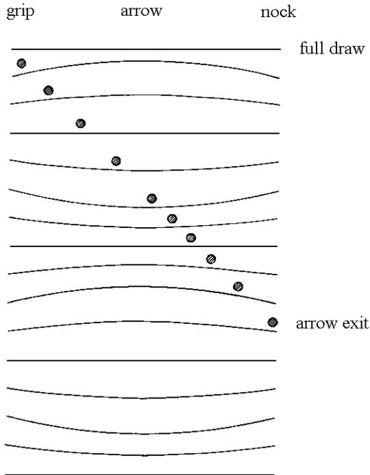
Figure 1: Illustration of archer's paradox (after Klopsteg [3, page 182 ]). Schematic representation of shapes of arrow during its passage of the bow, based on evidence from speed-flash. photography.
