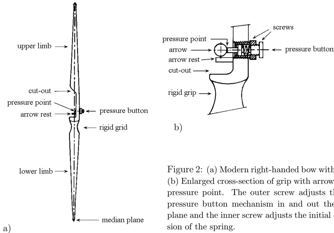
Figure 2: (a) Modern right-handed bow with cut-out. (b) Enlarged cross-section of grip with arrow rest and pressure point. The outer screw adjusts the whole pressure button mechanism in and out the median plane and the inner screw adjusts the initial compression of the spring.
